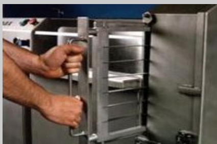
Fully interlocked knife frame giving shred length of 40/80/120mm or (25/50/75/100mm optional).
