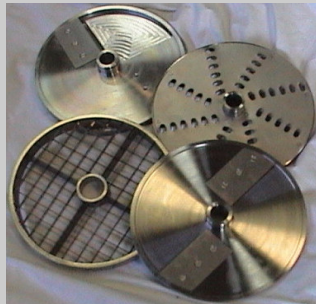
Stainless Steel "Type 316" cutting plates
